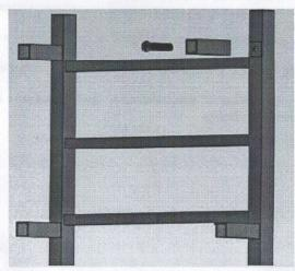
2. Measure and mark centre line and hole positions, drill holes on the wall, push wall plug into holes and fasten mounting pillar with wall.
